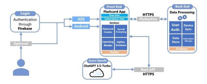
Figure 1: System Architecture
